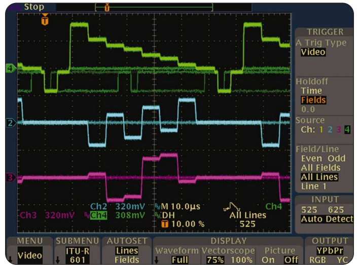
► Figure 7. TDS3SDI decoding of the 601 bit stream showing Y, P_b, P_r .
